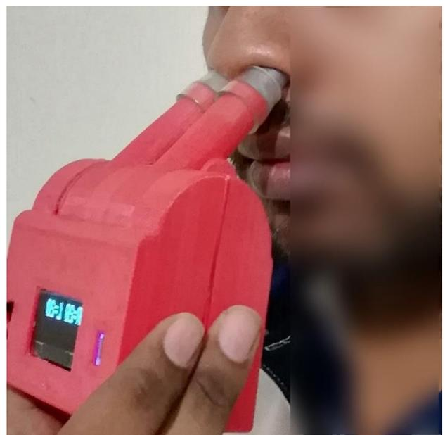
**Figure 6.** Using the NAMS for measurements
