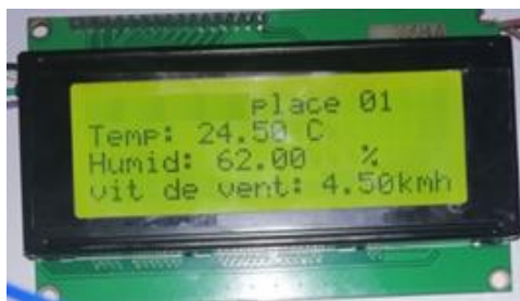
Figure 12. An example of the parameters displayed by LCD interface with Arduino
