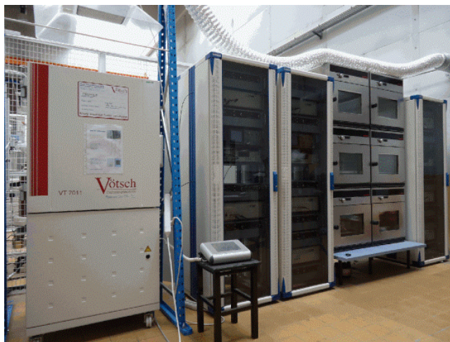
Figure 2. The experimental setup for accelerated tests
