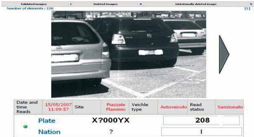
Figure 6: Example of license plate recognition screen page of the system.
