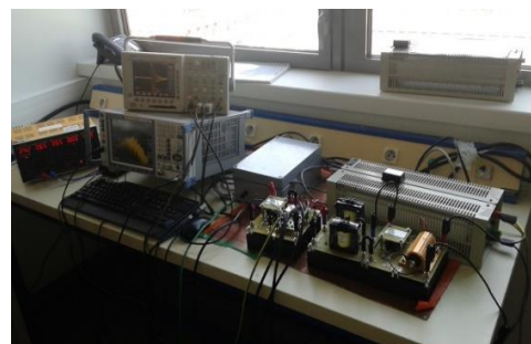
Figure 5. Test bench photograph: Power + LISN + Chopper "buck" + Load ( L = 2 \times 500 \mu\text{H} , C = 8 \times 22 \mu\text{F} , R = 100 \Omega ) with an electronic oscilloscope and a spectrum analyzer
