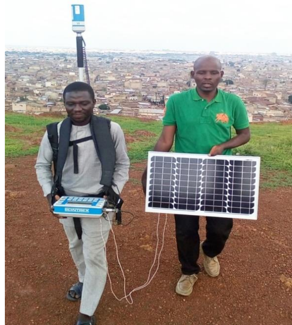
Figure 2. Magnetic data acquisition on dala hill
