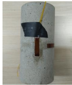
Figure 1. Strain gauge paste diagram
