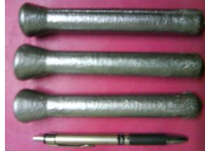
Figure 2. Hybrid composite gravity casting samples
