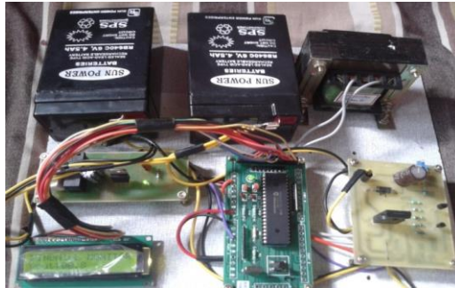
Figure 7. Power converter circuit board
