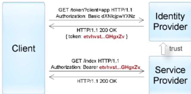
Figure 3. An example of authenticating an "active" client using a token transmitted via a support scheme
