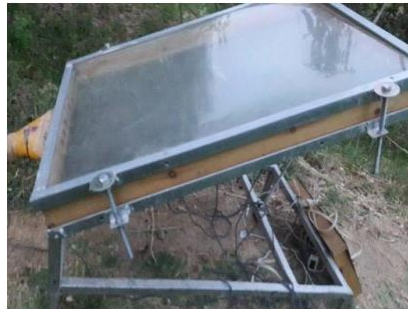
Figure 3. Single-glaze of solar collector
