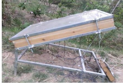
Figure 1. Solar collector realizes for the experimental study
