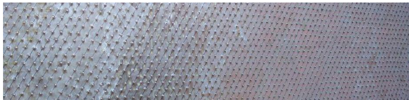
Figure 4. Photograph of spherical ball roughened absorber
