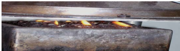
Figure 4: 'Zero Flame' treated MDF exposed at heat flux 65 \text{ kW/m}^2 .
