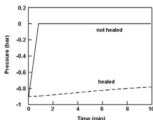
Figure 6: Vacuum decay recording during healing check tests.
