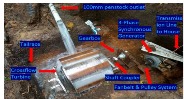
Figure 20. Mechanical system overview
