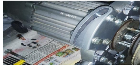
Figure 6. Modified 24V 500W 3-Phase synchronous generator
