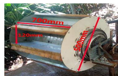
Figure 5. Fabricated mechanical crossflow turbine
