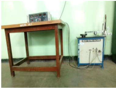
Figure 1. Ducom pin-on-disc apparatus for wear test
