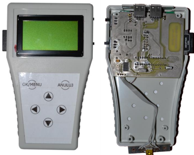
Figure 1. Air density measuring device
