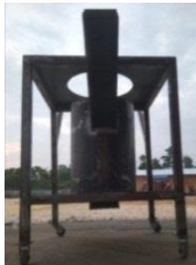
Figure 3. Updraft type biomass gasification furnace
