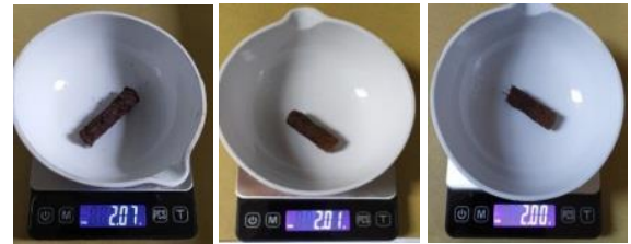
Figure 7. Sample mass characteristic testing of bio-pellets
