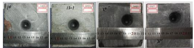
Figure 9. Erosion effects under different jet flow pressure
