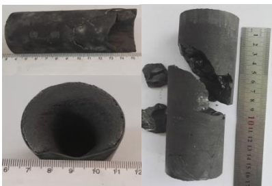
Figure 8. Coal breakage effect of abrasive gas jet
