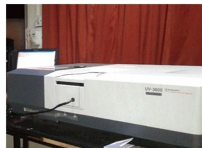
Figure 1. UV-3600 Shimadzu spectrophotometer with interfaced UV-Win lab software
