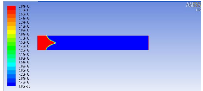
Figure 2. The CH_4 mass fraction
