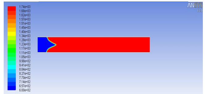
Figure 3. The adiabatic flame temperature contour
