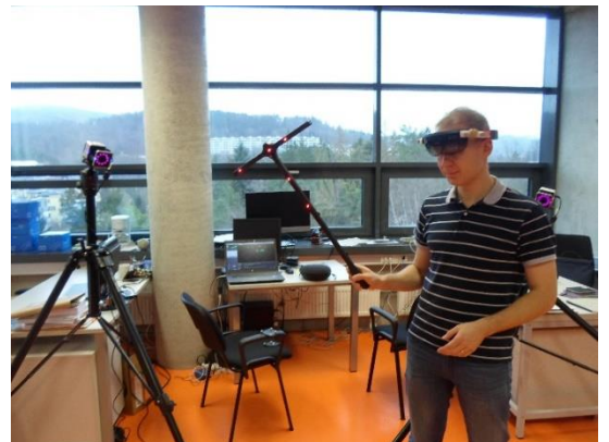
Figure 2. Calibration of the Vicon Motion Tracker
