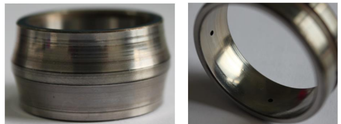
Figure 12. The morphology of the inner and outer rings
