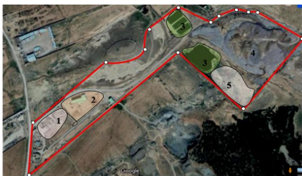
Figure 5. View and limitations area of the Batna landfill center: 1-administrative block, 2- sorting block, 3-leachate ponds, 4-waste lockers, 5 –extension ( https://maps.google.com/map )
