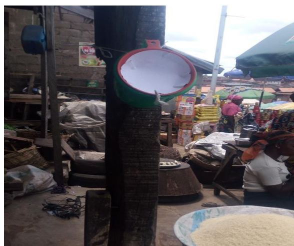
Figure 2. Improvised particulate collector before exposure
