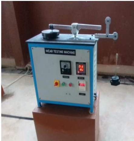
Figure 1. Wear test apparatus
