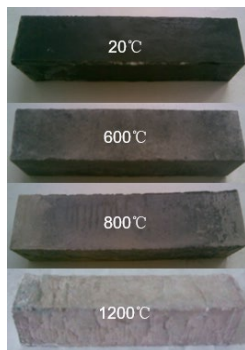
Figure 15. Appearance and color change of AASC samples exposed to high temperatures
