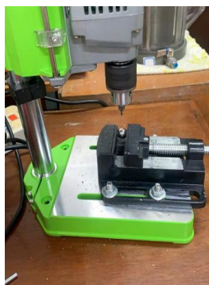
(a) Drilling holes in the steel ball
