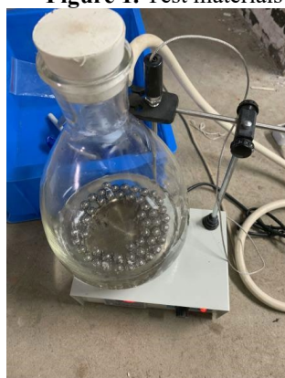
(b) Suction filtration of phase change steel ball
