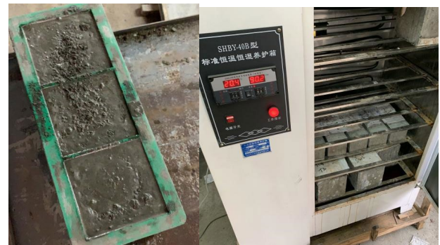
Figure 3. Preparation and maintenance of concrete test blocks
