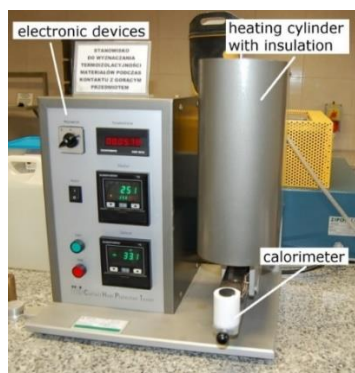
Figure 4. Experimental stand for measuring resistance to contact heat
