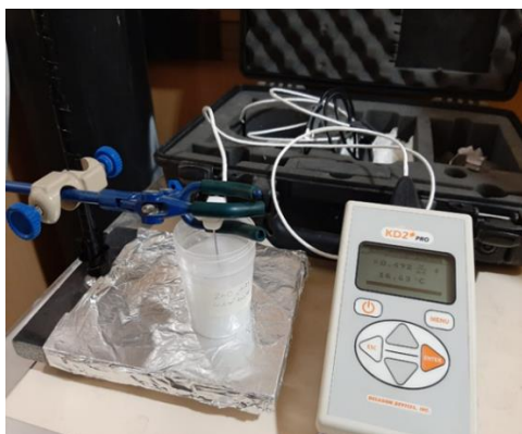
Figure 1. Thermal conductivity measuring of ZnO/DW nanofluids by KD2 Pro
