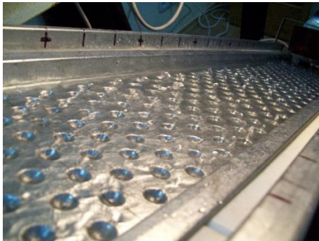
Figure 5. Features of water flow along the profiled tray T20 at G = 0.143 kg/s
