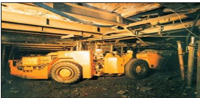
Figure 1. Typical LHD machine in a blasting gallery mine
