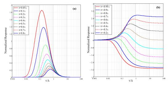
Fig.8. Half-sine Excitation Normalized Response for the 10 Channels Vs.  $T/\Delta$ . Where, A: Off-Time Response, B:On-Time Response
