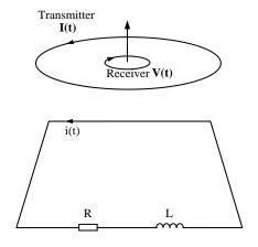
Fig.2. Free Space Loop Coil Response Model
