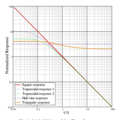
Fig.6. Initial Value of On-Time Response
