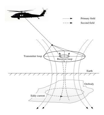
Fig.1. TD-AEM Operating Principle
