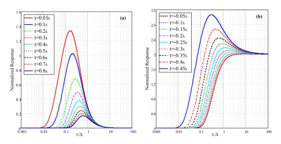
Fig.7. Triangular Excitation Normalized Response for the 9 Channels Vs. T/Δ. Where, A: Off-Time Response, B: On-Time Response
