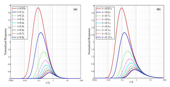
Fig.9. Trapezoidal Excitation Normalized Response for 9 Channels Vs.  $T/\Delta$ , Where A: Off-Time Response, B: On-Time Response
