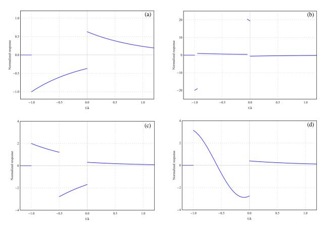
Fig. 5. Pulse Responses of Different Excitations in the Time Domain, Where Part A Is Square Excitation Response, Part B Is Trapezoidal Excitation Response, Part C Is Triangular Excitation Response, and Part D Is Half-Sine Excitation Response.
