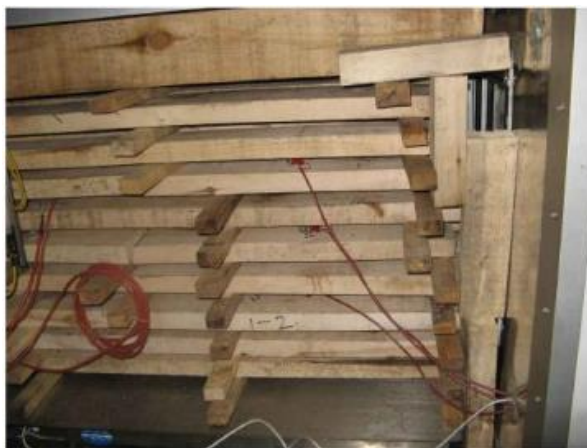
Fig.4. The Sensor Layout of Wood Carbonization Test
