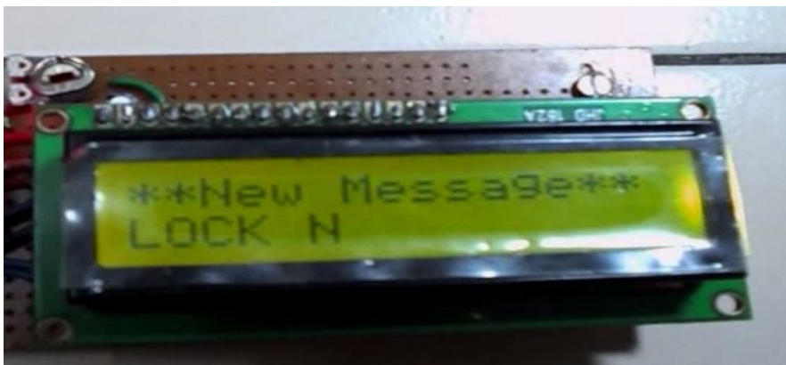
Fig.7. SMS received for activating the LOCK
