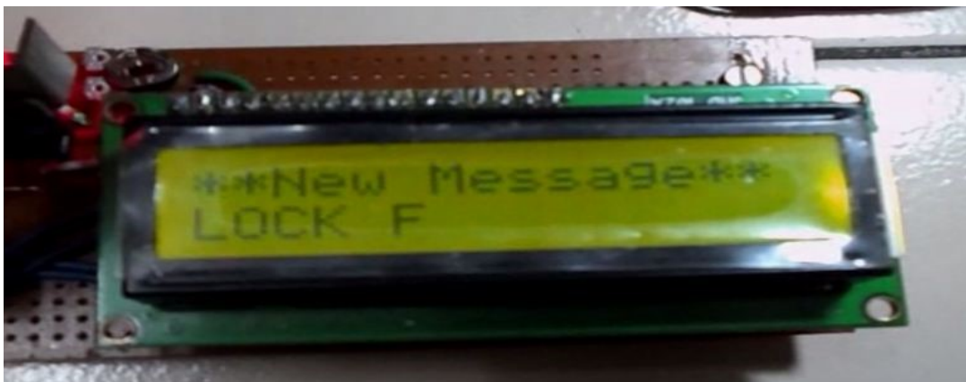
Fig.16. Sending Command to turn off the Lock
