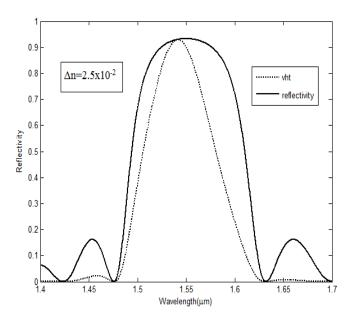
Fig.1. Reflectivity Profile with Wavelength for Hyperbolic-tangent Apodized Function, and Compared with Ideal Relfective Profile
