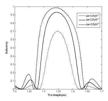
Fig.6. Comparative Study of Reflectivity Profile for Rised-Cosine Apodization Function for Different Refractive Indices
