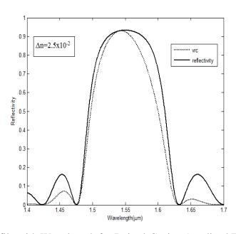
Fig.2. Reflectivity Profile with Wavelength for Raised-Cosine Apodized Function, and Compared with Ideal Reflective Profile
