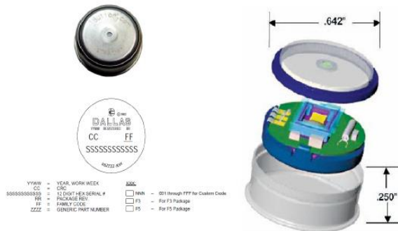
Figure 2. The Button-Thermochron, section of the internal components
