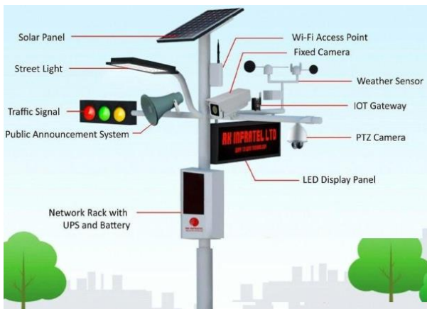
Figure 5. Smart electric poles equipped IoT gateway
