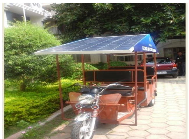
Figure 18. Fabricated model of proposed solar assisted ER
