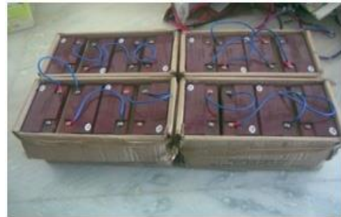
Figure 7. Traction Batteries – 4 x 12V 20Ah
