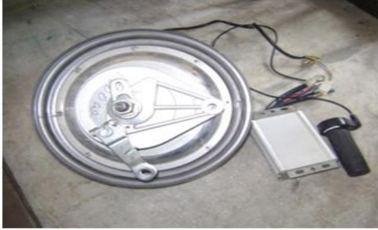
Figure 5. Permanent magnet brushless DC wheel hub motor with accelerator unit
