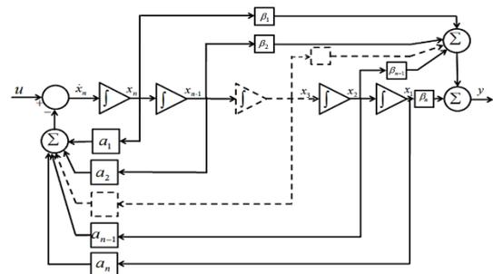
**Figure 1.** Block diagram representation of  $n^{\text{th}}$  order linear dynamical system
