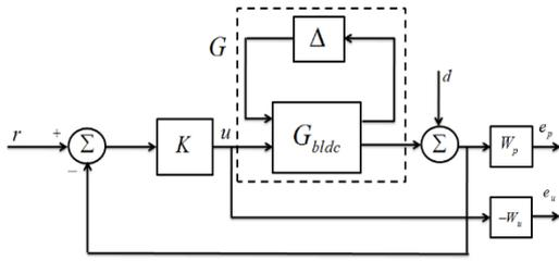
**Figure 10.** Closed loop structure of BLDC motor
