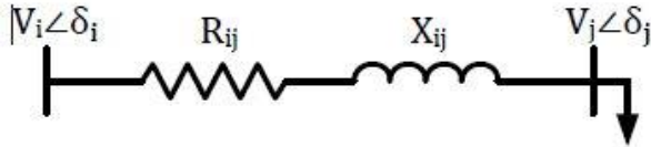
Figure 1. Radial distribution system with two-bus
