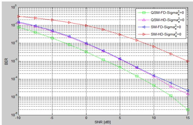
**Figure 7.** Comparison of QSM and SM System in FD and HD at  $\sigma_e^2 = 0$
