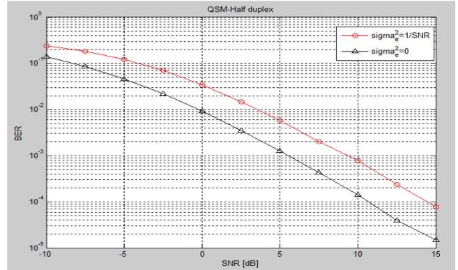
Figure 4. BER of QSM based HD
