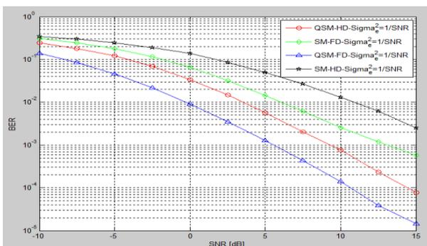
**Figure 8.** Comparison of QSM and SM in FD and HD at  $\sigma_e^2 = 1/SNR$
