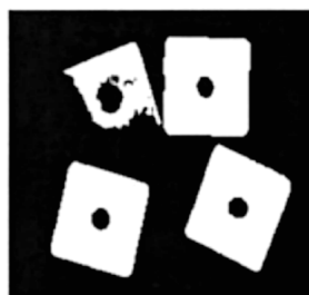
Figure 5-d. – Algorithme de Ridler
