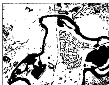
Figure 7-d. – Algorithme de Ridler
