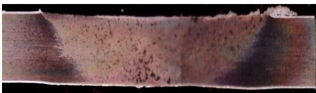
Figure 12. Macro structure of the welded joint
