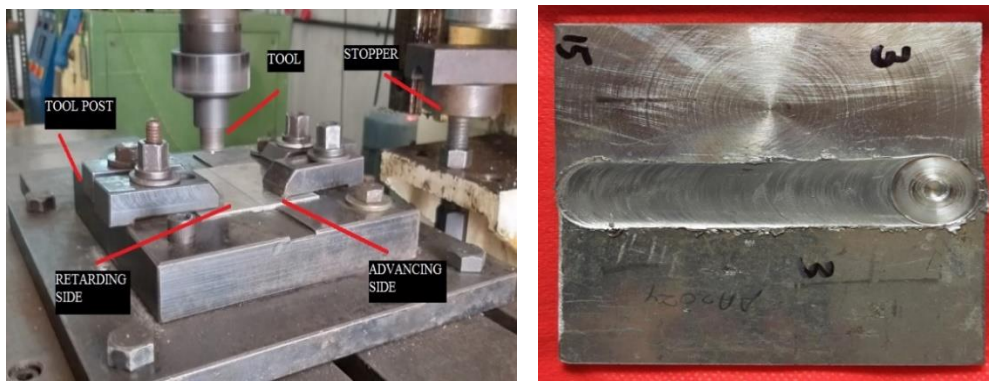
Figure 3. Layout of experimental setup & welded work piece
