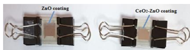
Figure 1. Completed DSSC's coated with ZnO and CeO 2 -ZnO composite
