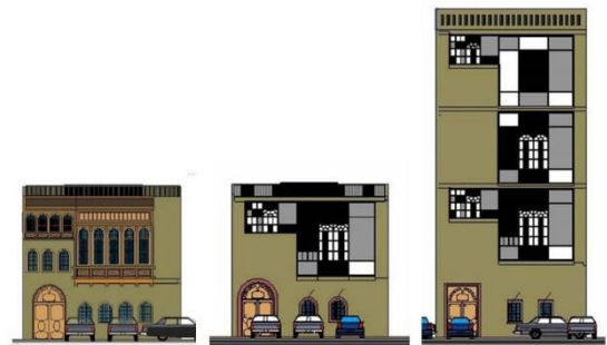
Figure 9. On the left, the illustration of the traditional wooden element in a typical example of two storey Baghdadi house. In the middle is a contemporary model with application of smart dynamic glazing elements using colours black, grey and white. On the right, the application of smart window/wall/balcony elements in a contemporary multi-storey building Source: author
