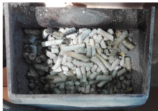
Figure 6. Ashes and unburnt hemp-hurd pellets in the fireplace of the wood stove at the end of the HEMP15GR combustion test
