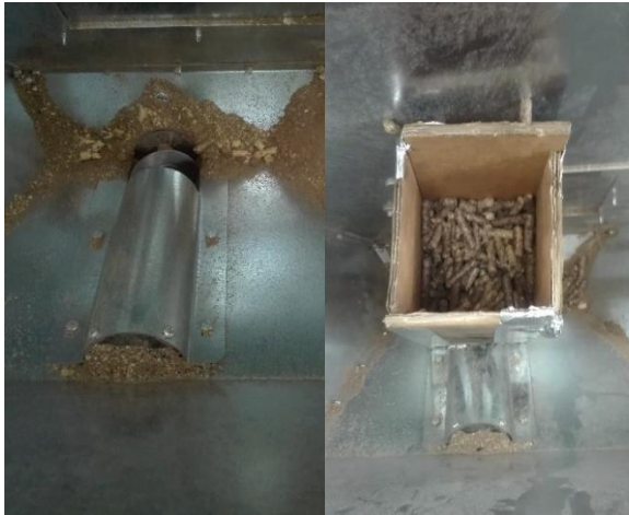
Figure 2. Standard hopper configuration (left) and modified hopper capacity (right)
