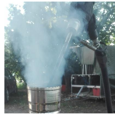
Figure 10. Smoke generation during the pellets ignition phase
