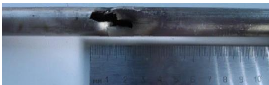
Figure 4. Photos of fragments of a tube with perforating damage (Balakovo NPP)
