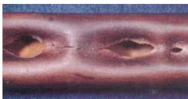
Figure 6. The damages of the cavitation character, described in Schwartz [2]
