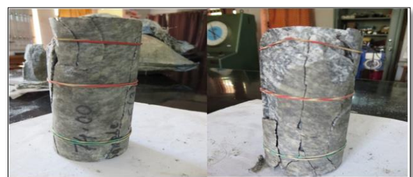
Figure 3. Fracture profile of Quartz Muscovite Schist after completion of UCS test
