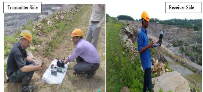
Figure 6. Range testing of communication modules at mine site
