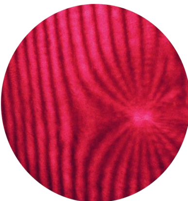
Moiré image of a glass blade with surface defects
