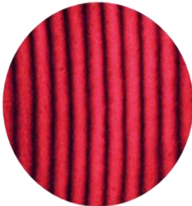
Figure 1. Moiré image of a glass blade without surface defects
