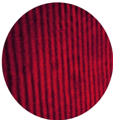
Figure 5. Moiré fringes characterizing the blade of a transparent plastic in its initial state inspected by the +1 order of the diffraction spectrum.
