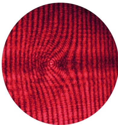
Figure 6. Moiré fringes characterizing a transparent plastic blade after creating a defect on its surface inspected by the order +1 of the diffraction spectrum
